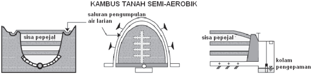
Figure 6 : Design of semi-aerobic landfill [14]
